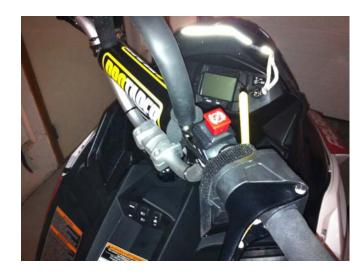
Cut the antenna tip to 2 cm's and place on the protective yellow cap.
