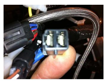
The Green and Brown Teth-Air wires Plug into this black plug. The gray wire is Not used and can be taped off or cut off.
