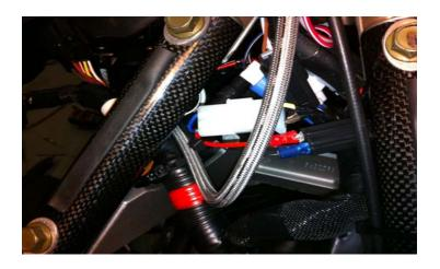
The power for the Teth-Air is available from the unused white AC accessory plug. The plug is an OEM design but accepts standard Molex 0.93 male pins and the nylon connector case even fits if the rounded edge is cut off
