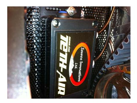
We decided that the best location was ahead of the exhaust side foot rest. The picture shown is with a Skinz mesh in in place which make it easy to mount. The LED indicator and push-button is easy to access with the side panel open. There is about 2 cm clearance to the belt drive. Use nuts and bolts with lock washers or Loctite so the Teth-Air can't vibrate loose. Wire-tie any loose wires to keep them out of the drive belt.
