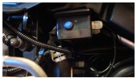
Start the machine to power up the Teth-Air. The engine should die in 1 second. This proves the operation of the system. Now re-start the engine while holding the blue button (or push and hold within 1 second of starting). The engine should remain running with the LED solid green, this will be the By-Pass Mode. Release and press the button a second time with the tag near-by and the Teth-Air Receiver will scan and record the unique code of up to 6 Tags. Your Teth-Air is now programmed.
