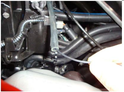
We also needed to bring up a wire for this connection. We used the tubing again to draw up a 24 inch wire that we had found in our scrap drawer. The brown wire from the Teth-air can be separated from the 5 wire insulated sheathing and brought to this plug if you do not want to run your own wire. Again, we used the tubing to pull the wire.
