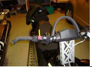
Below is the final installation with split loom installed on the exposed wiring.
