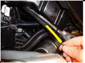
Next, locate the tube as it comes through above the motor. Stick the antenna tip (with cover installed) into the tube for a snug fit.
