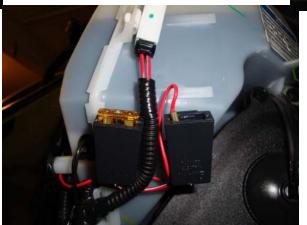
BRP provided a nice place to hook up for power. Our yellow wire was extended with this red wire to the AUX, fuse holder. We used a blade connector and plugged right on. ideally a light fuse could be installed and used to power the Cordless Teth-Air.
