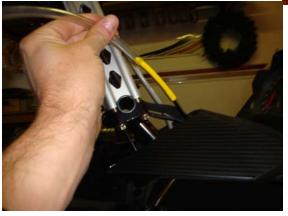
Slowly pull the tubing back out and this should bring the antenna wire up to the riser.
