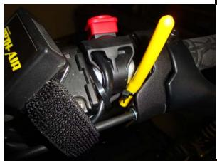
The yellow antenna cover must be vertical and near the wrist where the transmitter is worn. The pink shrink tubing can be removed if desired.
