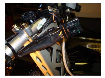
After covering the wires with some split loom to protect it, (top left) it was time to make the final connections. We used a 3 position terminal strip (bottom right) to connect the wire from the handle bar connector to the brown Teth-Air wire. We used another scrap wire (in split loom) to connect the white wire and the green wire to ground. We used the bolt for the side panel strap for the ground. (Top right.)
