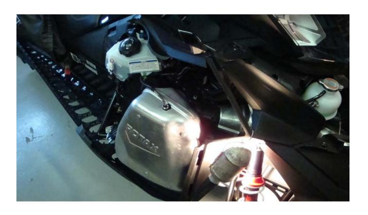
After much thought, we decided that the best mounting location was on the air box. We found sticky back industrial strength Velcro to be the best solution to avoid drilling holes in the air box. We used 2 inch wide product that is available at most hardware stores.
